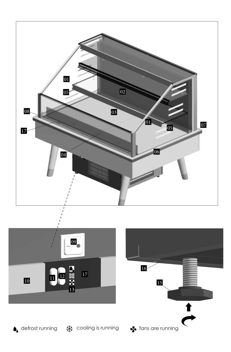
glass panes outside 01 glass shelf 02 floor display 03 battle plate inside 04 load limit line 05 decorative panel 06 impact protection 07 air intake grille 08 light switch LED (optional) 09 thermostat controller 10 program keys 11 button forward-back 12 display icons ₩ 4, % 13 temperature display 14 adjustable feet with thread M10 15
