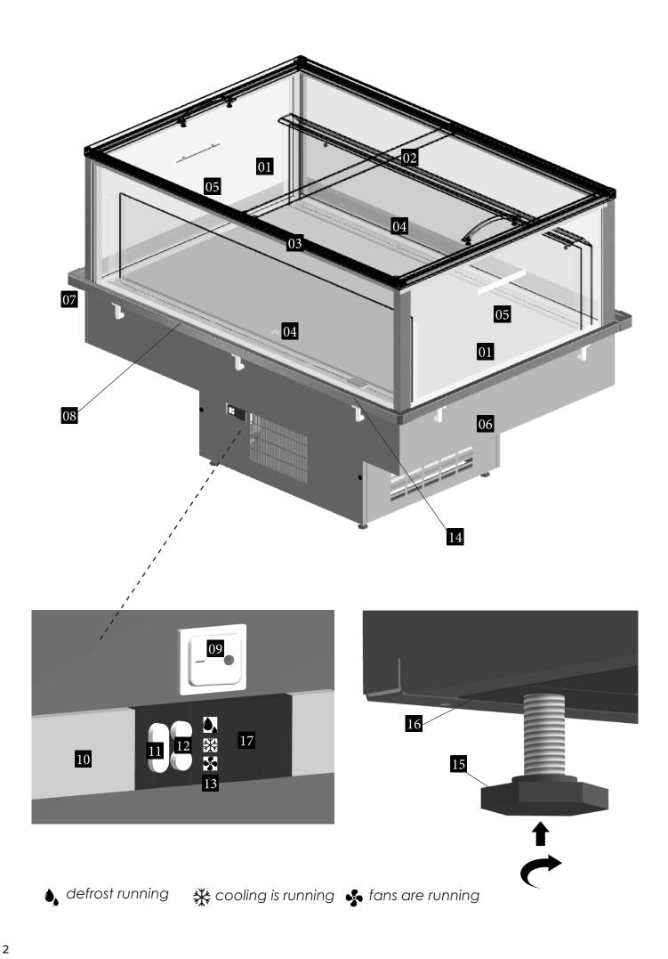
glass panes outside 01 sliding glass lid 02 floor display 03 baffle plate inside 04 load limit line 05 decorative panel 06 impact protection 07 air intake grille 08 light switch LED (optional) 09 thermostat controller 10 program keys 11 button forward back 12 display icons ₩ 4, % 13 temperature display 14 adjustable feet with thread M10
