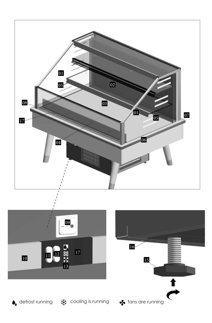
glass panes outside 01 glass shelf 02 floor display 03 battle plate inside 04 load limit line 05 decorative panel 06 impact protection 07 air intake grille 08 light switch LED (optional) 09 thermostat controller 10 program keys 11 button forward-back 12 display icons ₩ 🔥 🐝 13 temperature display 14 adjustable feet with thread M10 15
